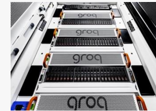
9 Groq nodes, 8 GroqChip/node (TSPs)
